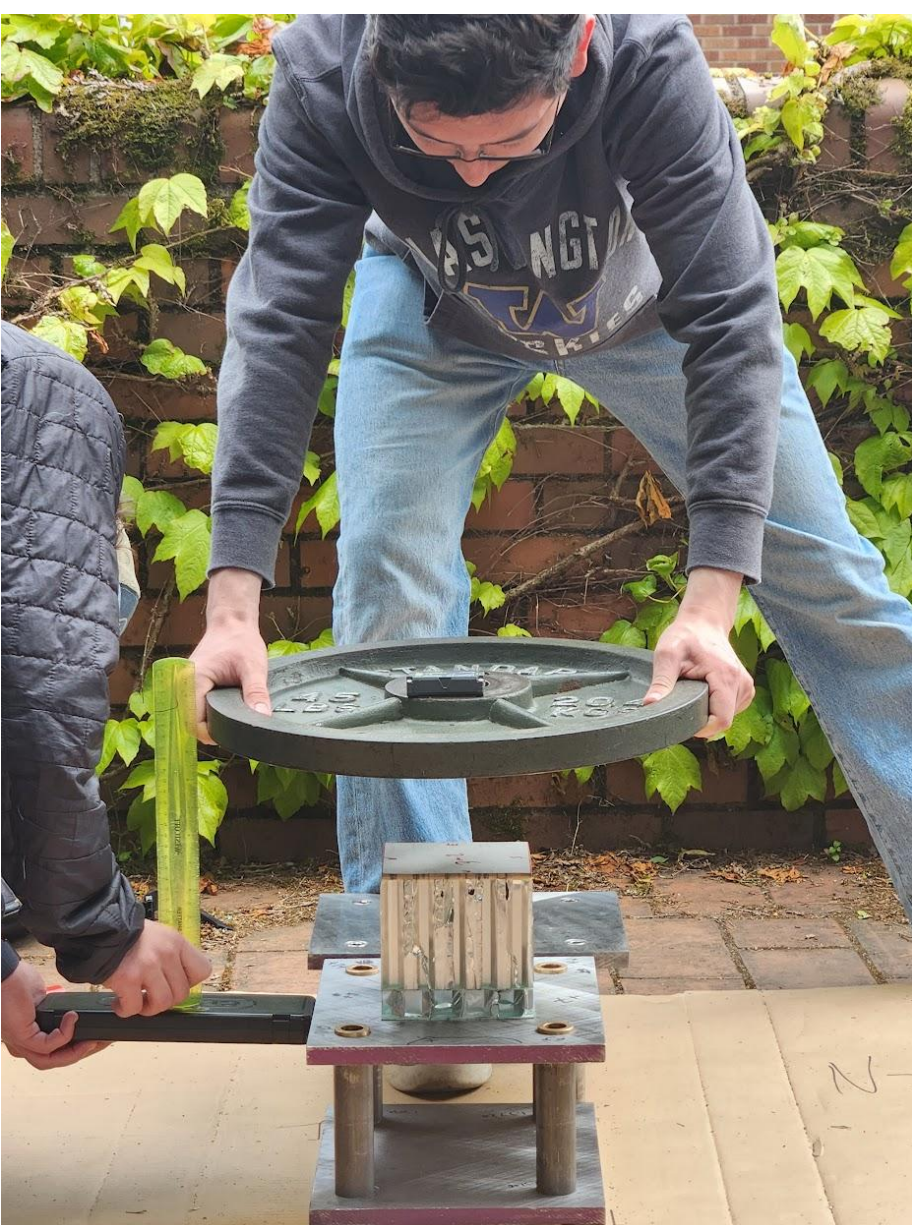
Figure 5: Sample on Impact Frame
