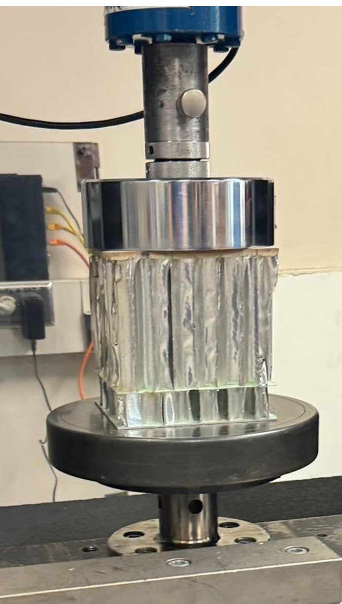
Figure 3: Sample in Instron Load Frame
